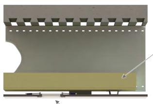
4" LED Downlight suspended from gypsum board
