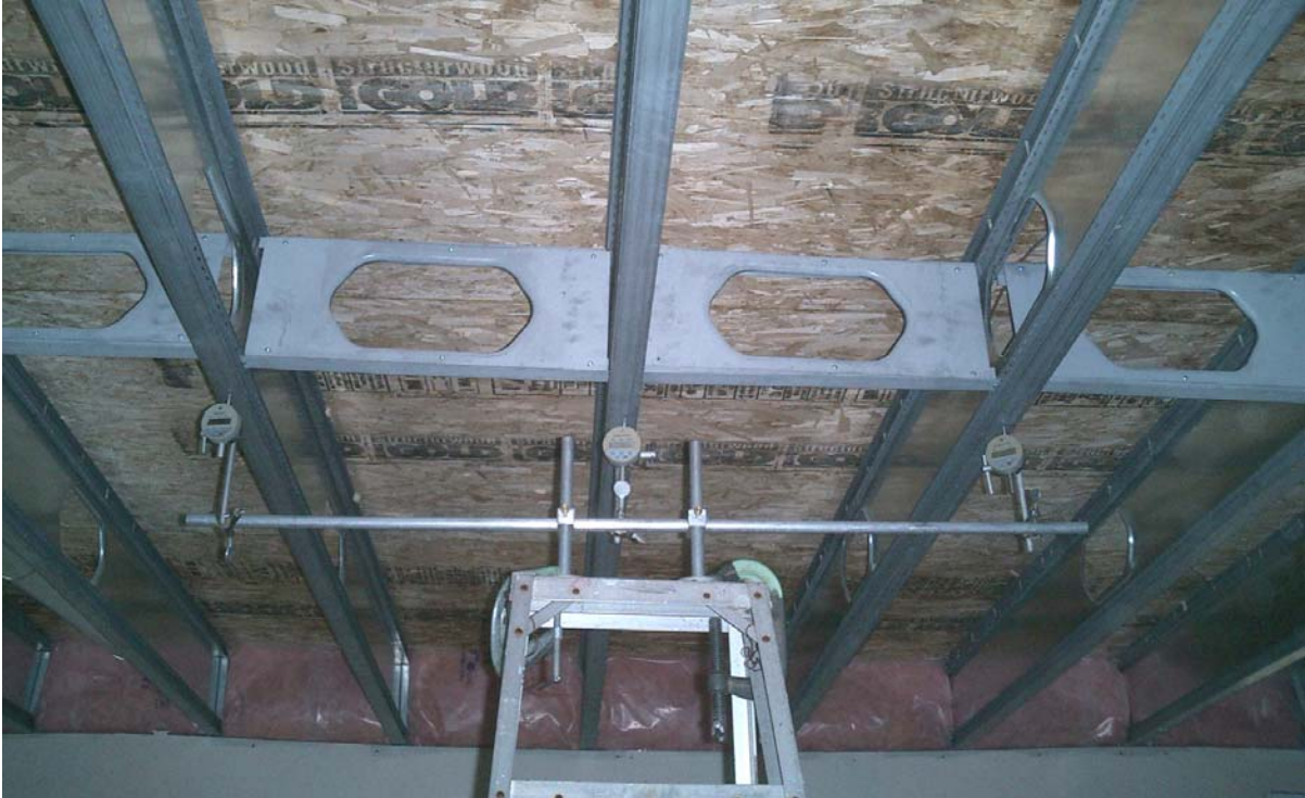
Figure 3.6: Deflection measurement setup of static test
