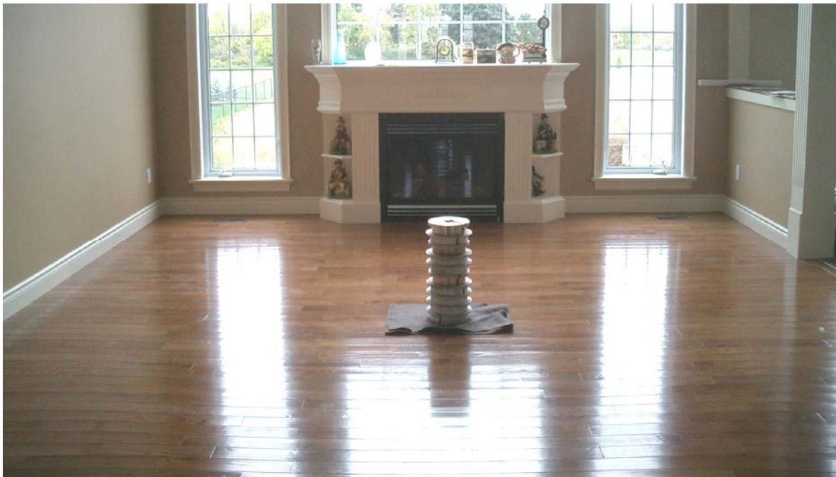
Figure 3.5: 1-kN weight setup of static test
