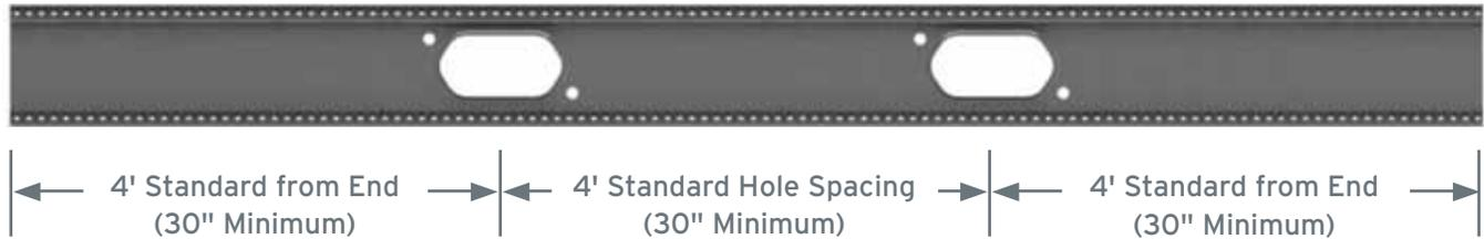
Composite TotalJoist web holes are fully customizable and can come in any of the following arrangements:
